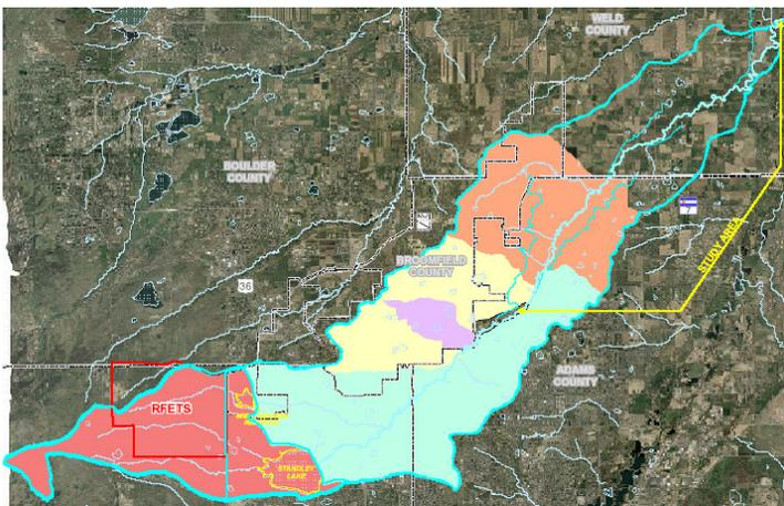
Shaded areas identify boundaries of stormwater master plans completed in the watershed in the past. Yellow lines show the area of focus for Lower Big Dry Creek Hydrologic Study. Northeast shaded area (in peach) will be the study area for the update to the Big Dry Creek North Area Tributaries Outfall Systems Plan.
